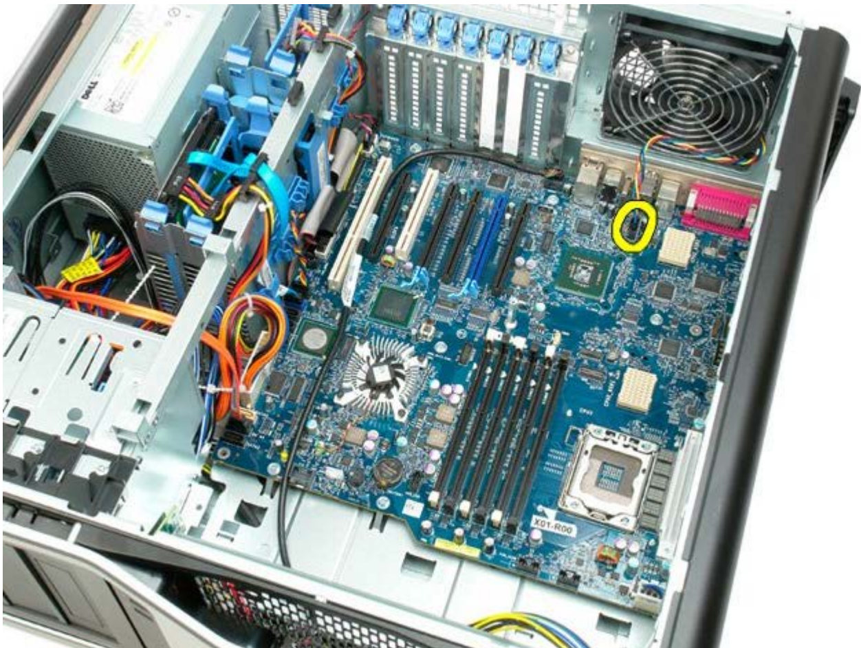
9. Frakobl frontpanelets lyd kabel.
